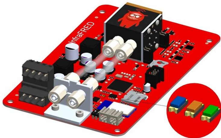
Illustration 31: Status LED Multi-Gas Sensor InfraFRED
